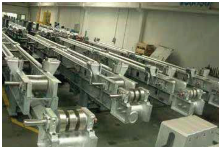
Pre-assembled Roller Tables.
