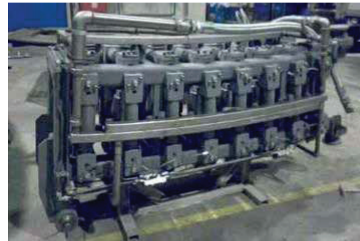
We fulfill leakage and flow test procedures for CCM segments.
