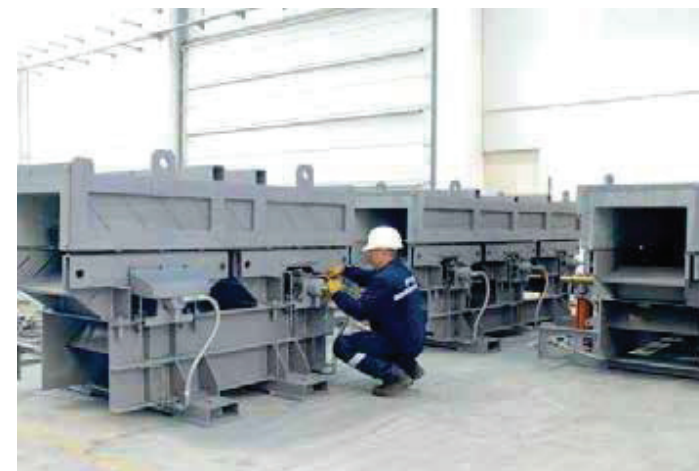
■ Final checks of a roller table with insulated covers.
