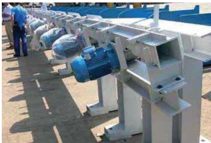
■ Inlet Roller Table assembled.
