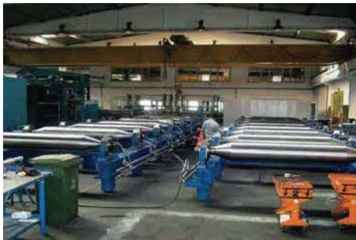
Roller table for Hot Strip Mill.
